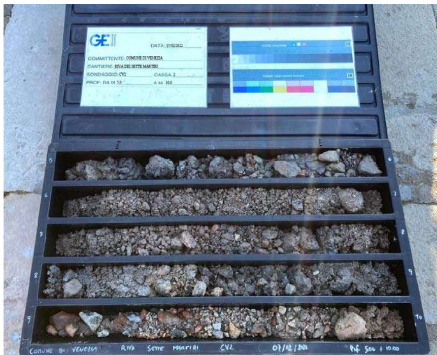
SONDAGGIO CV2 – CASSA 2 – DA 5,0 A 10,0 M
