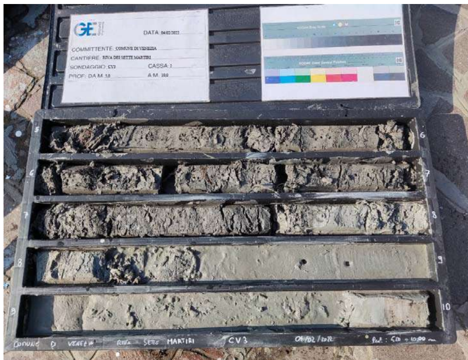
SONDAGGIO CV3 – CASSA 2 – DA 5,0 A 10,0 M
